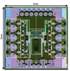
[Chen et al, ISSCC 2013] Peak Tx efficiency 17.4%. Maintains > 7% efficiency while transmitting 6 Gbps (16-QAM)
