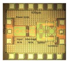
[Chen et al, ISSCC 2011] 18.6dBm 60GHz Power Amplifier in 65nm
