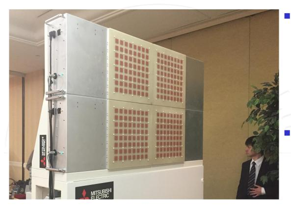
A very large number of antennas, much larger than the number of user beams; form "beams" from the basestation to users simultaneously
