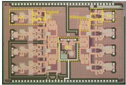
4 Elements (Separate TX/RX) 137 mW Total (Rx or Tx mode)
