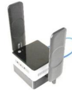
Prototype COSMOS SDR Node (Medium)
