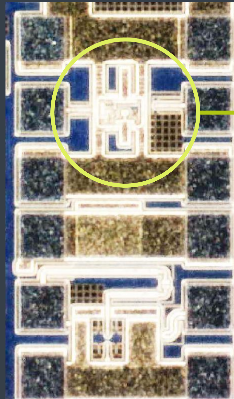
First-ever mm-wave bandwidth CCII
